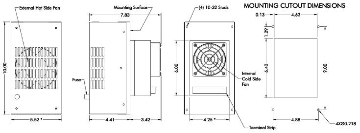
\* Dimension does not include hardware, insulation. Dimensions: Inches, Mounting hardware and gasket included but not shown.
